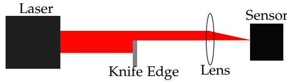
Figure 4: Schematic setup of a knife edge measurement. The power within the laser beam is measured while the knife edge is moved across the beam.
